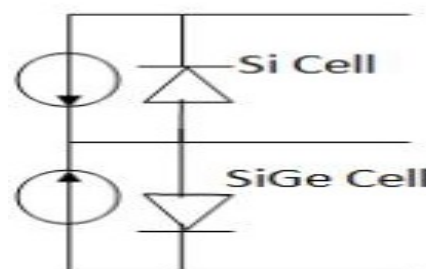
Figure 4: Equivalent circuit of Si-Si:Ge tandem solar cell.
